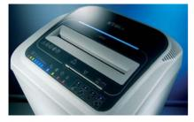
Touch Screen Panel Just touch the controls to activate the machine functions. Keep your finger on the "Forward" control for 5 seconds and the machine functions continuously for 30 seconds when transparent material needs to be shredded. A light comes on when the blades need to be oiled.
